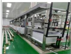
The equipment is mainly used for replacing silver paste with copper plating such as silicon wafers of photovoltaic cells.
