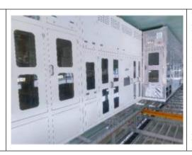
The mass production line of PV battery piece metalization is mainly used for copper plating such PV batterv as silicon to replace silver paste. It can also be used for certain technical paths such as BC, HJT, TOPCan.
